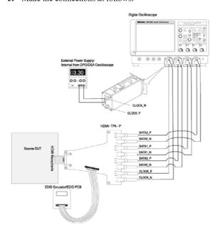
6. Ensure that your signal in the oscilloscope display is similar to the sample signal. Click View Waveform to display a sample of the expected signal. If the displays are not similar, go back and check your configuration and connections.
